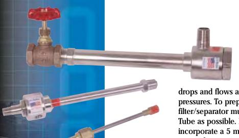
With our models ranging from approximately 6" to 13" long, Vortex Tubes are a very compact source of refrigeration and spot cooling capability. They are designed to utilize a filtered compressed air supply of 80 - 110 PSIG. Pressures lower than 80 PSIG will still provide some cooling, but temperature
