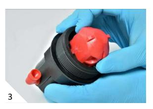
• Insert the Float halfway into the Body [1], insert the Clamping Stem into the Rolling Seal groove of the Body; make sure that it is inserted in the direction of the arrow [2]. Push the Float and the Clamping Stem together downwards into the Body until they are locked [3].
