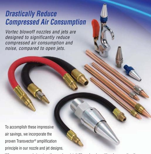
When compressed air enters the nozzle or jet, it fills a chamber with only one exit path – a thin annular orifice. As air passes through this orifice, it accelerates to 1000 ft (304.8 m) per second, entraining free surrounding air as it exits. The result is airflow volume up to 25 times more than supplied by the compressed air.
